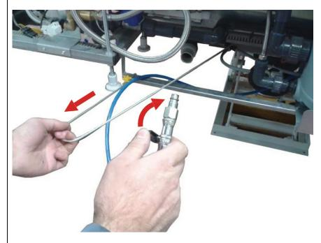
**To lower the bathtub**, connect the air tube on the bathtub to the compressor.
